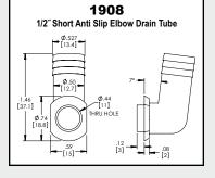
All drain tubes are molded in High Impact ABS (black) plastic.
